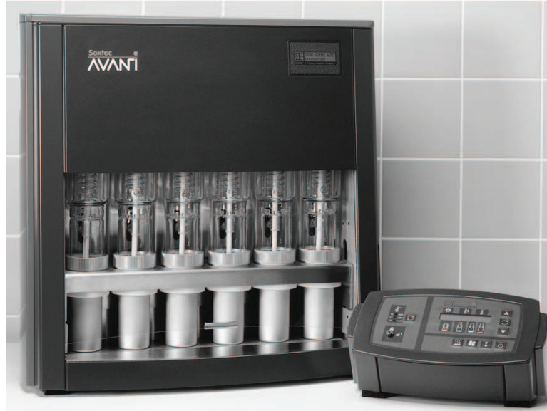
Figure 4.3 The Soxtec™ Avanti 2050 automated extraction system [8].
