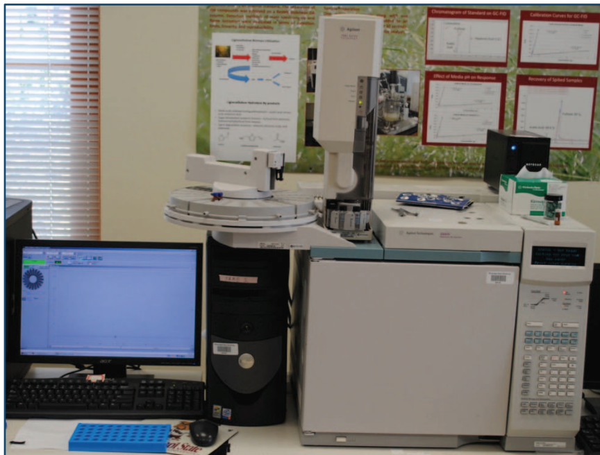
Figure B.16 Agilent 6890N gas chromatograph equipped with flame ionization detector (Agilent, Santa Clara, CA, U.S.A.).
