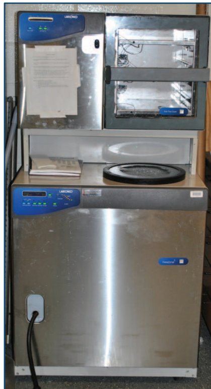
Figure B.6 Freezezone 6 Bulk Tray Freeze dry system (Labconco, Kansas City, MO, U.S.A.).
