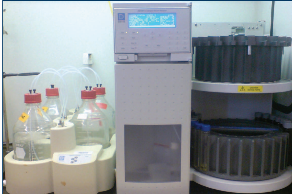
Figure B.7 ASE® 200 system equipped with a multi-solvent control system (Dionex, Sunnyvale, CA, U.S.A.).
